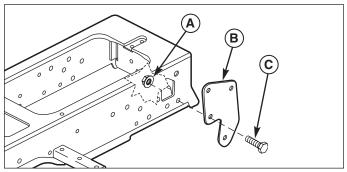
Figure 1. Install Side Brackets
